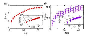
FIG. 4. Plots of the gap radius (a) and height (b) vs time. The insets show that *r* and *h* grow with power laws consistent with  $t^{1/3}$ . Fitting to these parameters for *L*, we find values of  $(2.5 \pm 0.1) \times 10^6$  J/kg and  $(2.31 \pm 0.02) \times 10^6$  J/kg, respectively (see Supplemental Material for details [22]).
